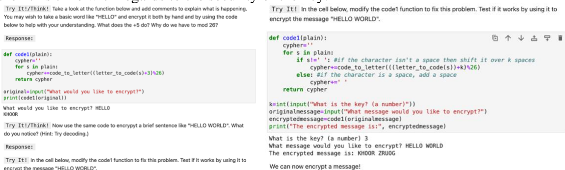
Figure 2. Left: A section of the scaffolded ‘Cryptography’ activity in which students are guided through programming the encryption process of the Caesar cipher. Students should discover that the provided code does not consider spaces when encrypting and that this will affect the decrypting process. Students are then asked to alter the code to fix this problem. Right: An example of a solution code to encrypt a message.
